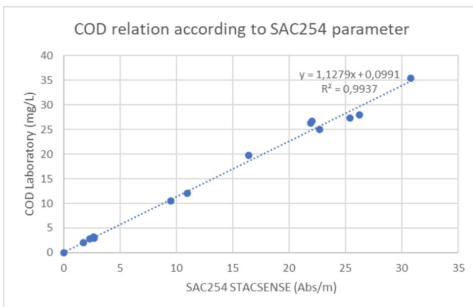
The linear regression line proposes a new relationship between the UV absorption at 254 nm (CAS254) and the CODeq -> CODeq = 1.1279 \* CAS254 + 0.0991.
